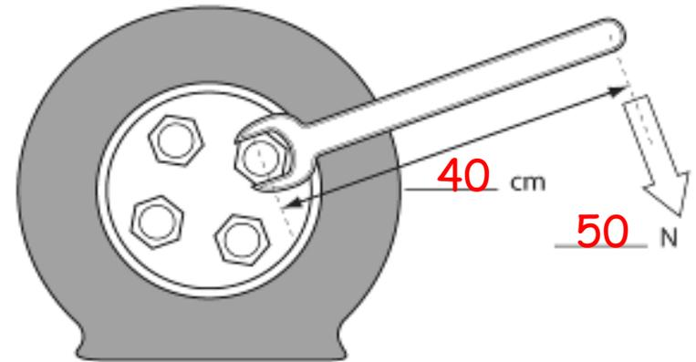
**Moment of the force (Nm) = Force (N) x Distance from pivot (m)**
