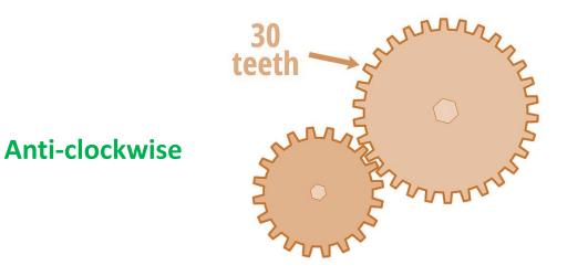
7. In the gear system shown above, the 30 tooth cog rotates once every 5 seconds. The smaller cog has 15 teeth. Calculate how long it will take to the smaller cog to complete one revolution.
