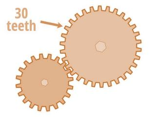
In the gear system shown above, the 30 tooth cog rotates once every 5 seconds. The smaller cog has 20 teeth.
