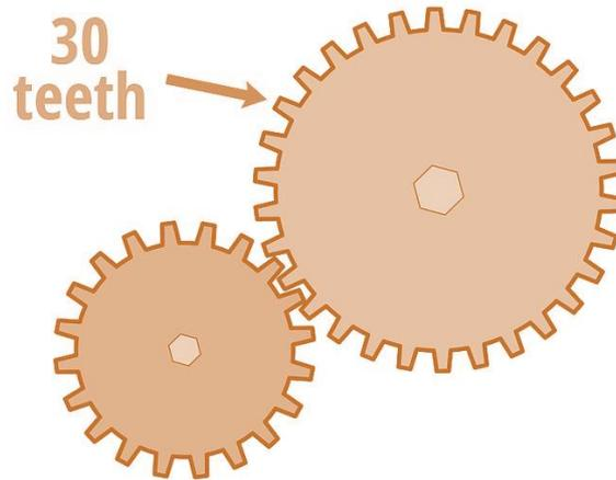
7. In the gear system shown above, the 30 tooth cog rotates once every 5 seconds. The smaller cog has 20 teeth. Calculate how long it will take to the smaller cog to complete one revolution.
