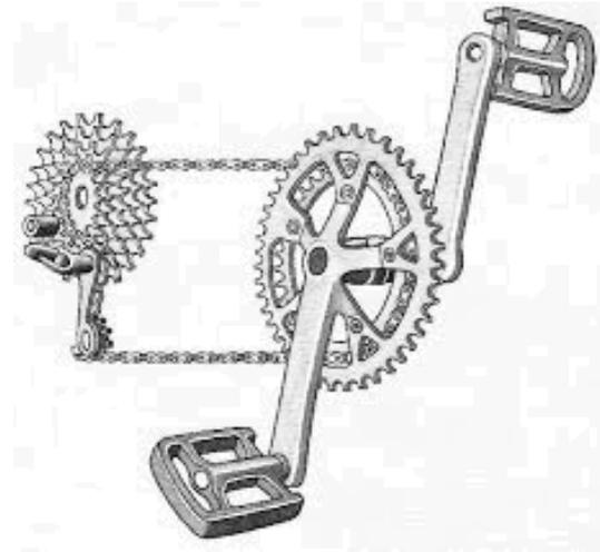
Sometimes gears are connected by a chain.
