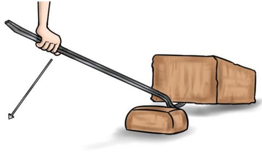
By pushing down on the crowbar the object is lifted upwards.
