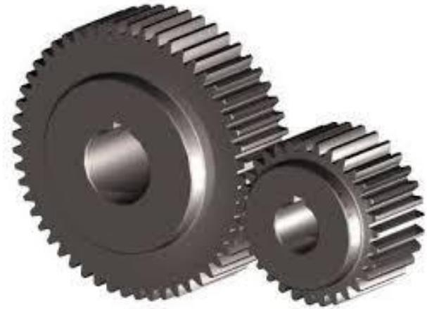
When the large gear rotates once the smaller gear may rotate many times.
