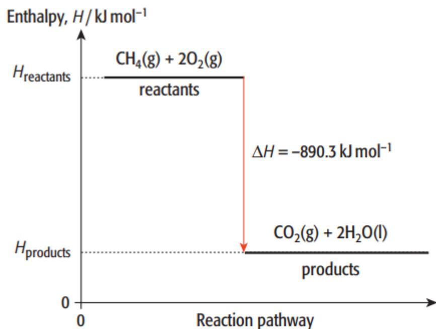
**Figure 6.3** Enthalpy profile diagram for the combustion of methane.
