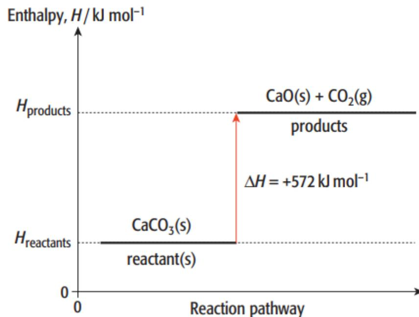
**Figure 6.4** Enthalpy profile diagram for the decomposition of calcium carbonate.
